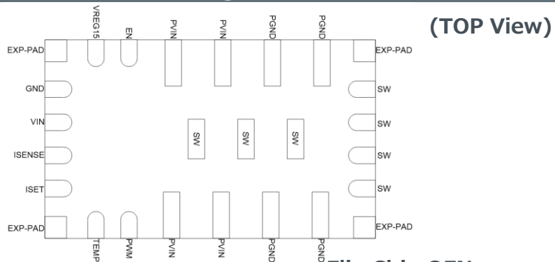
Flip Chip QFN (23pin, 5.0mm x 3.0mm)
